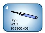
Wipe all liquid from the exterior of the AMPOULE and WAIT 30 SEC-ONDS for full color development (Fig. 4).
