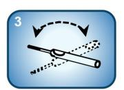
Mix by inverting the HARDNESS TEST AMPOULE back and forth to dissolve the reagent (Fig. 3).
