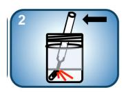
Place the tip of the HARDNESS TEST AMPOULE into the angled hole in the bottom of the SNAPPING CUP. While applying downward pressure, break the tip of the AMPOULE by tilting the AMPOULE toward the far edge of the SNAPPING CUP.
