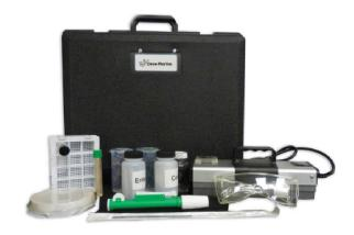
Ballast Water Test Kit-QC contains reagents and apparatus to test for presence of particular indicator organisms, that is, tests for Total Heterotrophic Bacteria, E.coli, and Enterococci. The tests available in Ballast Water Test Kit-QC are suitable and practical for onboard testing, and because the results are quantitative, the responsible crew member will have quick access to data on which to make an informed decision concerning the effectiveness of the ballast water treatment system.
