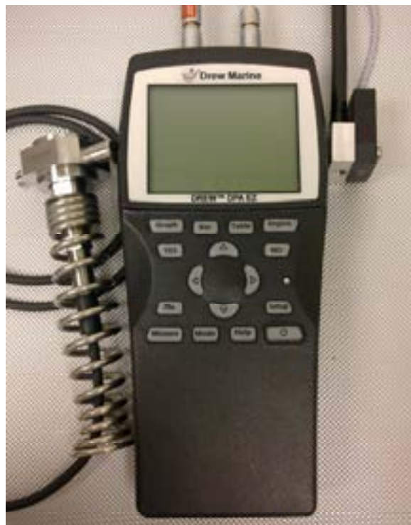
Drew DPA-EZ analyzer shown with Cylinder Pressure Sensor mounted in Thompson Adaptor
