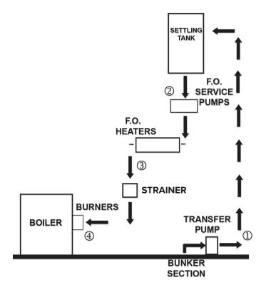
Recommended injection points for AMERGY 1000 combustion improver in typical steam propulsion fuel arrangement:
