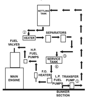
Recommended injection points for AMERGY<sup>®</sup> 1000 combustion improver in typical main engine fuel arrangement:
