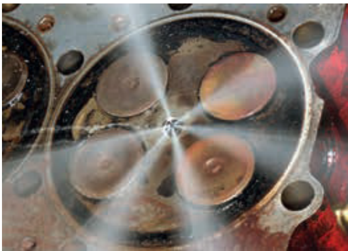
Poor spray pattern from blocked injector holes
