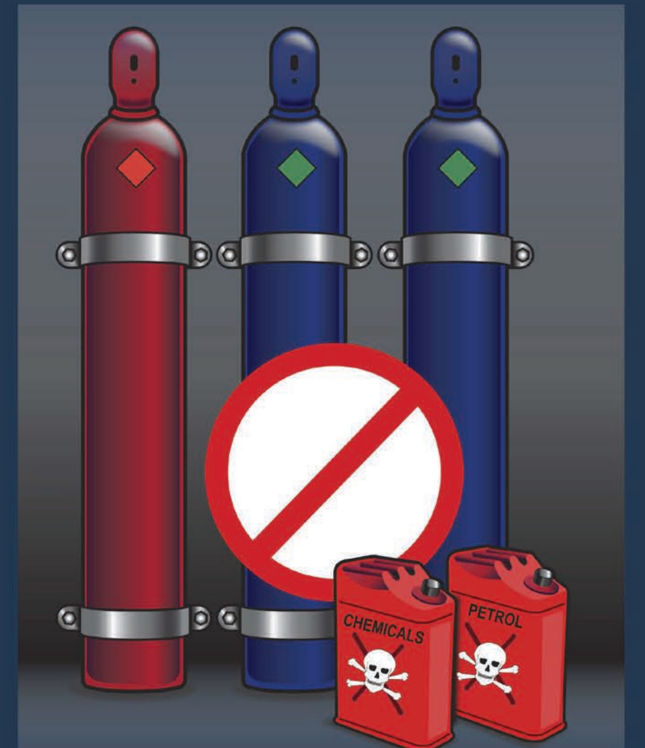
Do not store with combustible material. Do not store acetylene and oxygen cylinders together.
