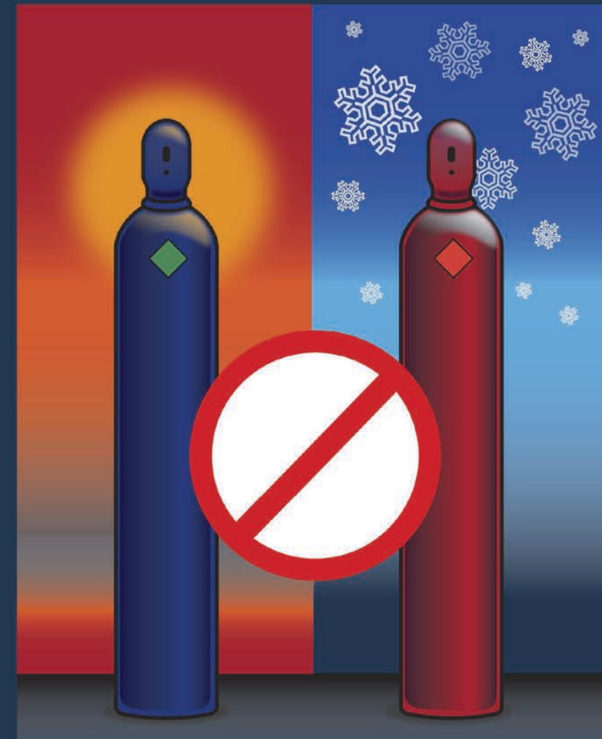
Never store cylinders in extremely hot or cold temperatures.
