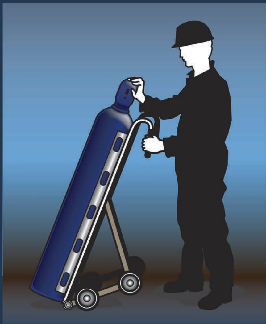
Transport cylinders in upright position. Replace valve caps when cylinders are not in use.
