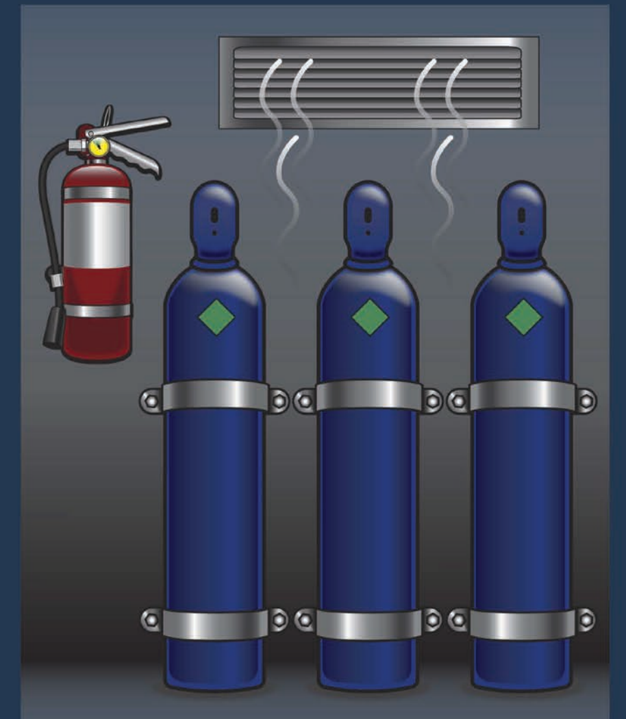
Store in separate compartment or room. Always provide ventilation. Always have a fire extinguisher nearby.
