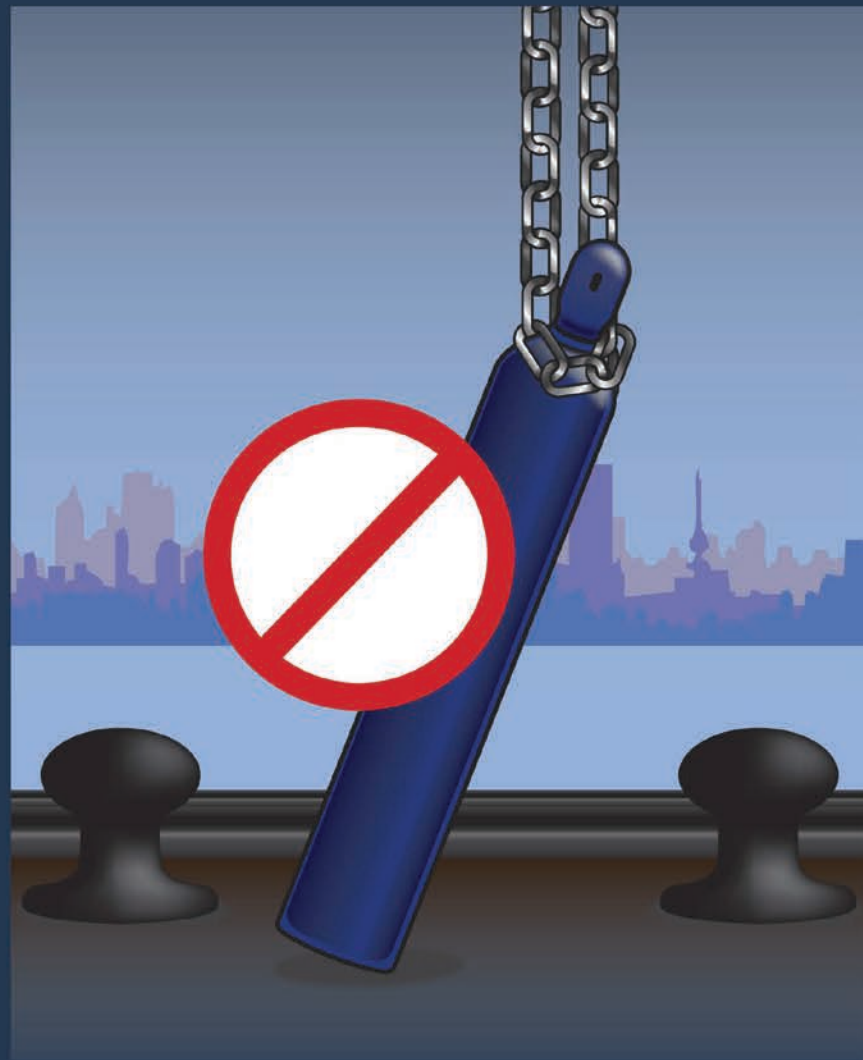
Do not lift by top valve or cap with slings, chains or magnets.
