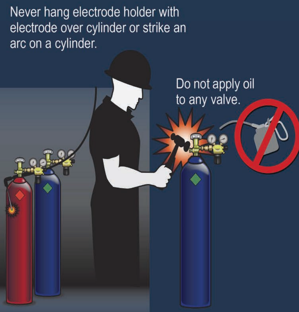
Never use a spanner or hammer to open or close the valve. Use hand pressure only.
